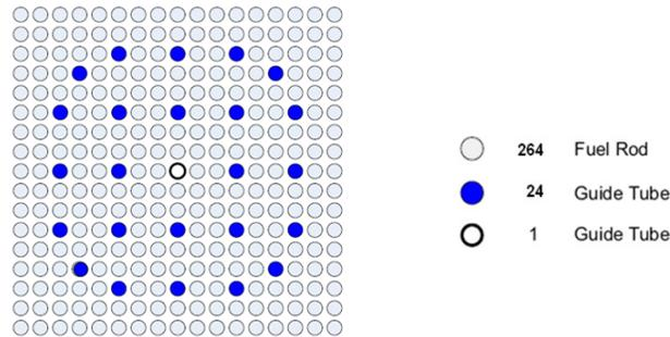
Figure 2 – Assembly fuel pattern.
