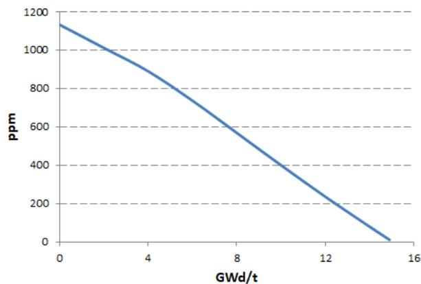
Figure 4 – Critical boron vs. burn-up at the equilibrium cycle
