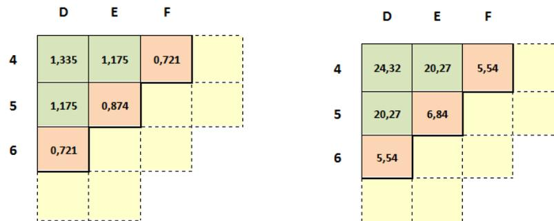
Figure 7 - Assembly 2-D average relative power fraction (left) and burn-up distribution (right) at MOEC.
