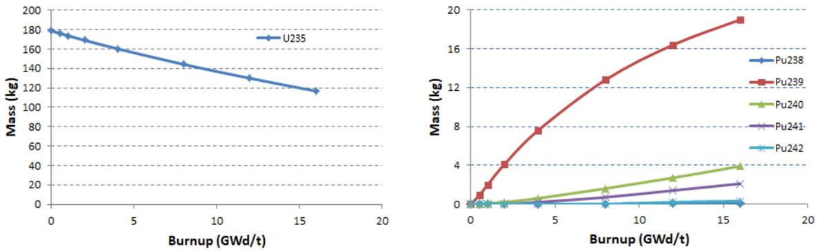
Figure 10 – Mass of <sup>235</sup>U (left) and of plutonium isotopes (right) vs. burn-up for the 1<sup>st</sup> cycle
