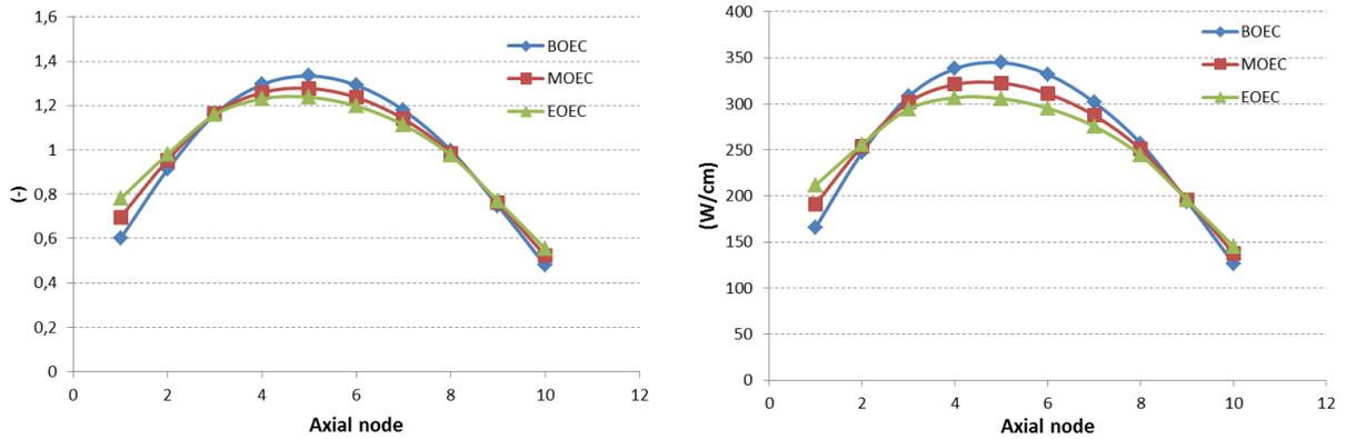
Figure 20 – MOX core: axial relative power fraction (left) and axial peak power distribution (right) at BOEC, MOEC and EOEC.
