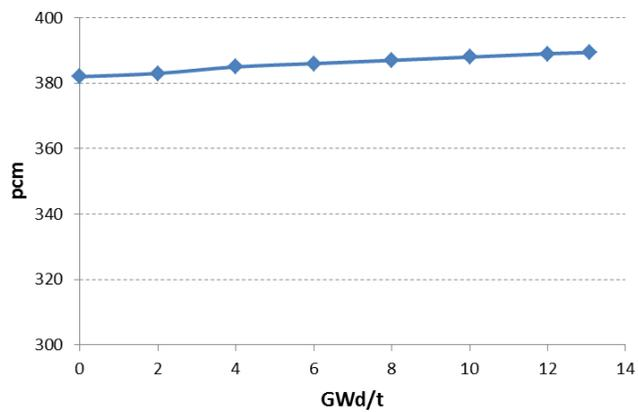
Figure 25 – MOX core: effective delayed neutron fraction vs. burn-up at the equilibrium cycle.
