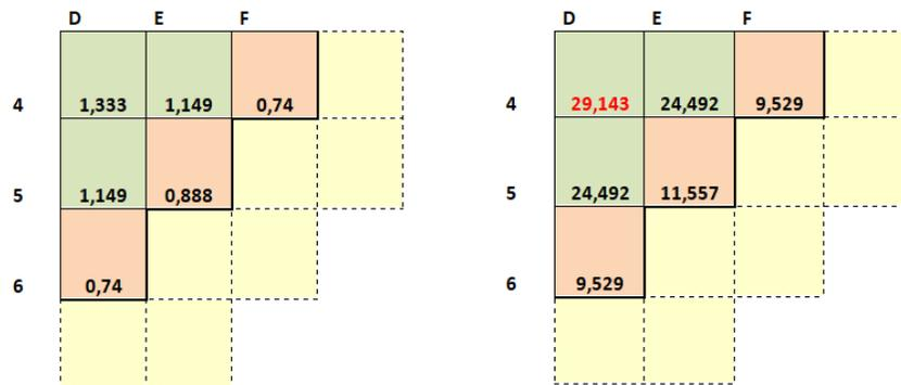
Figure 24- MOX core: assembly 2-D average relative power fraction (left) and burn-up distribution (right) at EOE.
