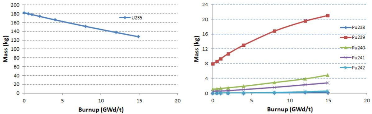
Figure 12 – Mass of <sup>235</sup>U (left) and of plutonium isotopes (right) vs. burn-up at equilibrium cycle.
