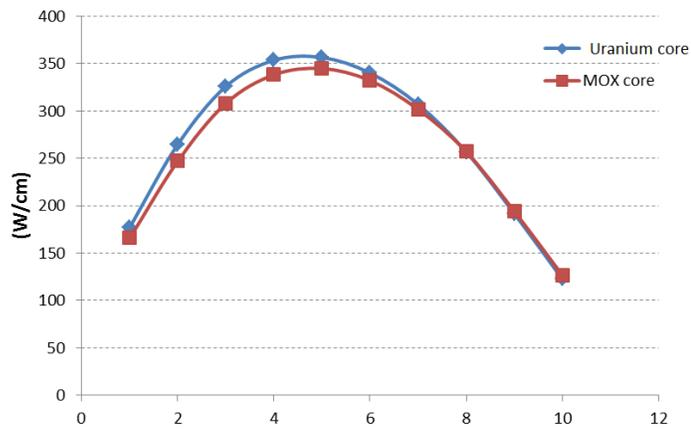
Figure 21 – Axial peak power distributions at BOEC for the MOX core and comparison with the trend for the UO<sub>2</sub> core.
