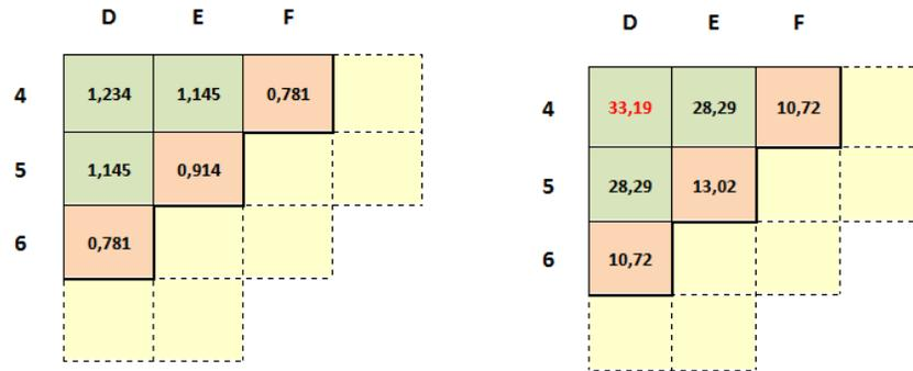
Figure 8 - Assembly 2-D average relative power fraction (left) and burn-up distribution (right) at EOEC.
