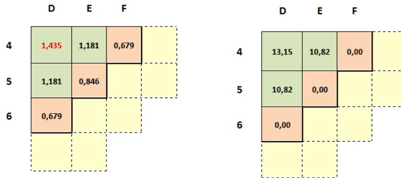
Figure 6 - Assembly 2-D average relative power fraction (left) and burn-up distribution (right) at BOEC.
