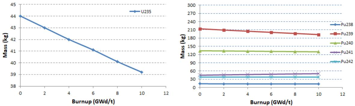
Figure 26 – MOX core: mass of  $^{235}\text{U}$  (left) and of plutonium isotopes (right) vs. burn-up for the 1<sup>st</sup> cycle.
