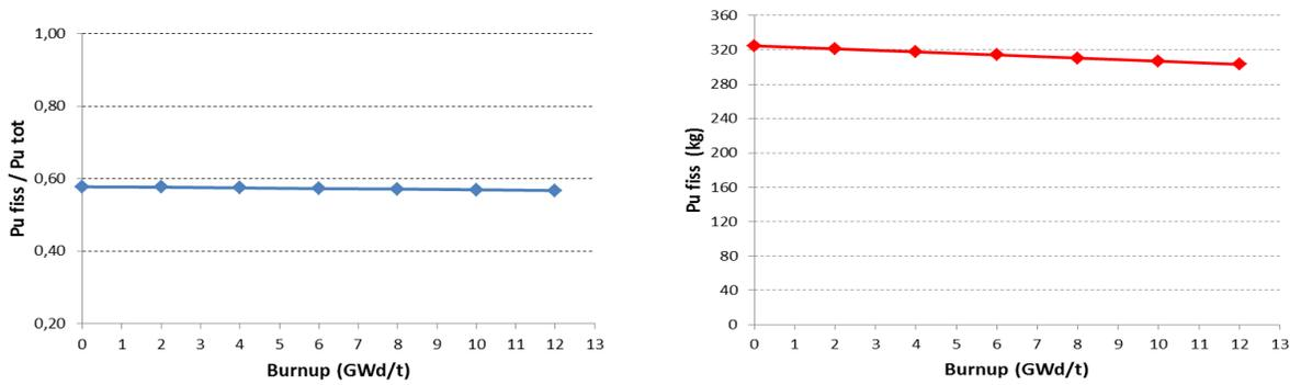
Figure 29 – MOX core: trend of the ratio  $Pu^{fiss}/Pu^{tot}$  (left) and of total amount of fissile plutonium ( $^{239}Pu+^{241}Pu$ ) (right) vs. burn-up at the equilibrium cycle.
