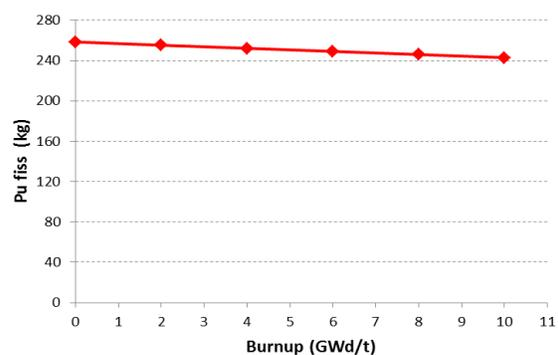
**Figure 28 – MOX core: trend of the ratio  $\text{Pu}^{\text{fiss}}/\text{Pu}^{\text{tot}}$  (left) and of total amount of fissile plutonium ( $^{239}\text{Pu} + ^{241}\text{Pu}$ ) (right) vs. burn-up for 1st cycle.**
