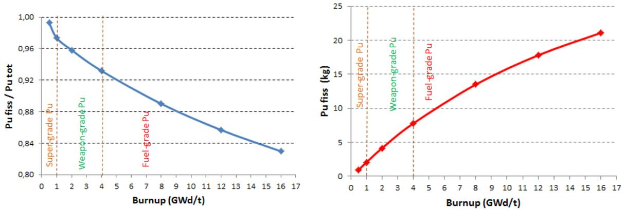
Figure 13 – Trend of ratio  $Pu^{fissile}/Pu^{total}$  (left) and of total amount of fissile plutonium ( $^{239}Pu+^{241}Pu$ ) (right) vs. burn-up for the 1<sup>st</sup> cycle.
