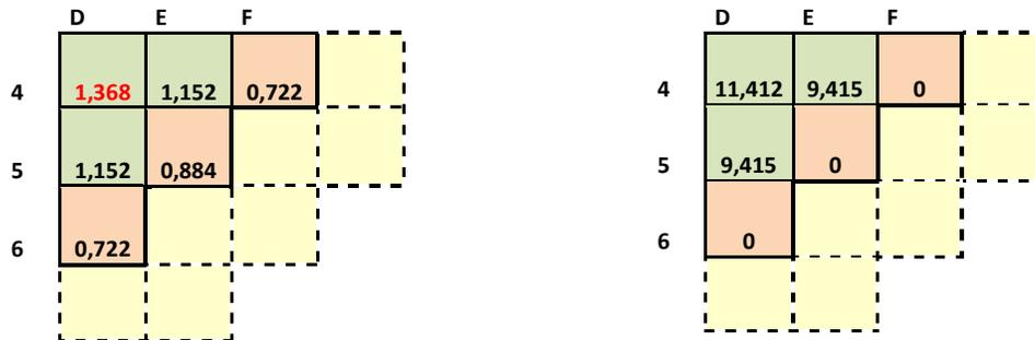
Figure 22- MOX core: assembly 2-D average relative power fraction (left) and burn-up distribution (right) at BOEC.
