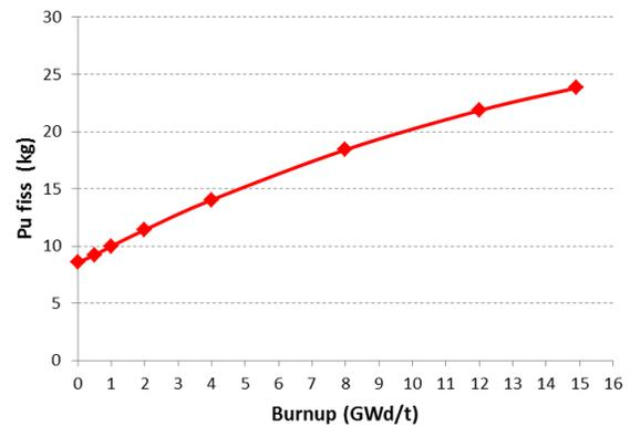
Figure 15 – Trend of ratio  $Pu^{fiss}/Pu^{total}$  (left) and of total amount of fissile plutonium ( $^{239}Pu+^{241}Pu$ ) (right) vs. burn-up at equilibrium of cycle.
