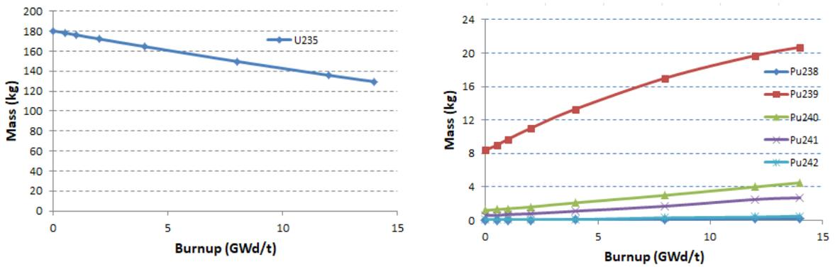
Figure 11 – Mass of <sup>235</sup>U (left) and of plutonium isotopes (right) vs. burn-up for the 2<sup>nd</sup> cycle.
