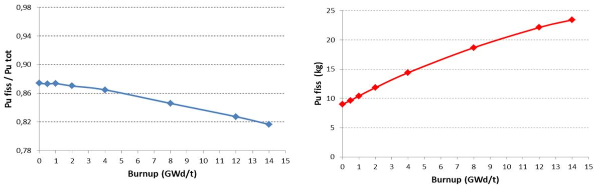
Figure 14 – Trend of ratio Pu<sup>fissile</sup>/Pu<sup>total</sup> (left) and of total amount of fissile plutonium (<sup>239</sup>Pu+<sup>241</sup>Pu) (right) vs. burn-up for the 2<sup>nd</sup> cycle.
