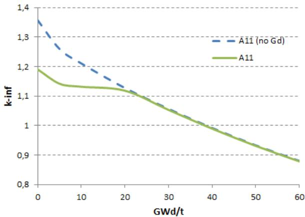
Figure 3 – Trend of reactivity along the first burn-up cycle for the fuel assembly  $A_{11}$ .
