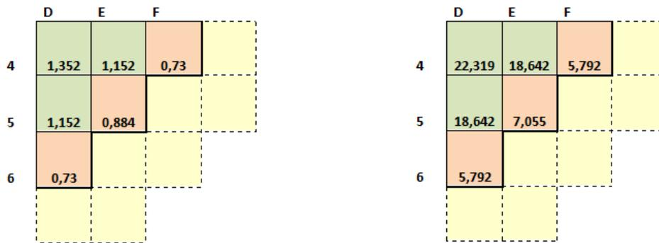
Figure 23- MOX core: assembly 2-D average relative power fraction (left) and burn-up distribution (right) at MOEC.
