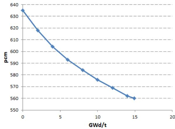
Figure 9 – Effective delayed neutron fraction vs. burn-up at the equilibrium cycle.
