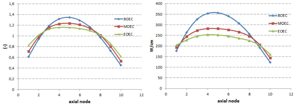
Figure 5 – Axial relative power fraction (left) and axial peak power distribution (right) at BOEC, MOEC and EOEC.
