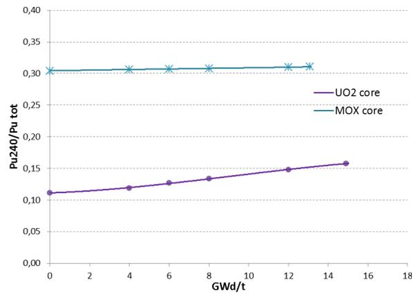
Figure 30 – Comparison of the ratio  $^{240}Pu/Pu^{tot}$  vs. burnup for UO<sub>2</sub> core and MOX core (equilibrium cycle).
