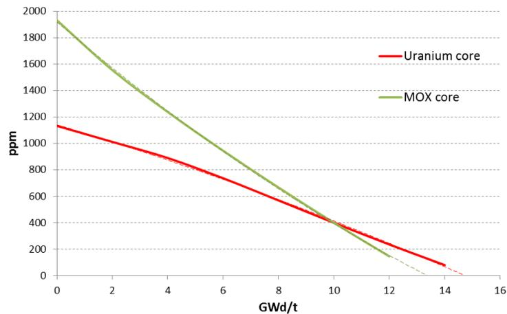
**Figure 19 – Trends of critical boron vs. burn-up at equilibrium cycle for the MOX core and comparison with the trend for the  $\text{UO}_2$  core.**
