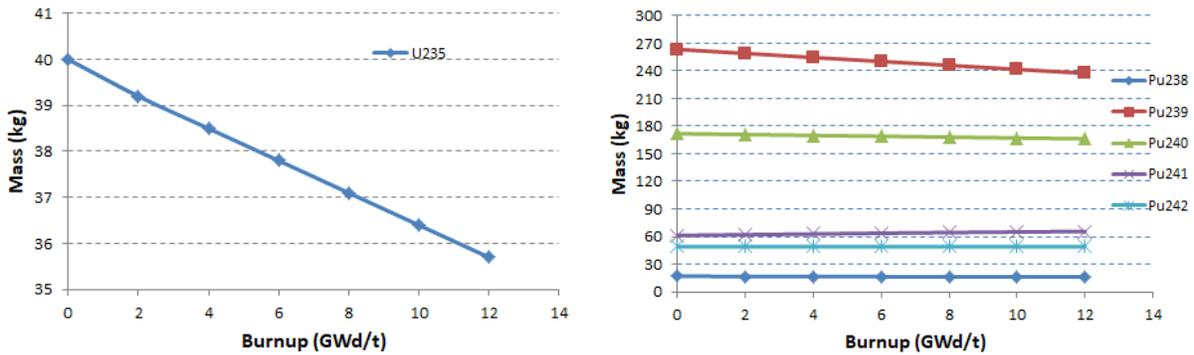
Figure 27 – MOX core: mass of  $^{235}\text{U}$  (left) and of plutonium isotopes (right) vs. burn-up at equilibrium cycle.
